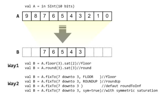
fixTo is strongly recommended in your RTL work, you don't need to handle carry bit alignment and bit width calculations manually like **Way1** in the above diagram.
