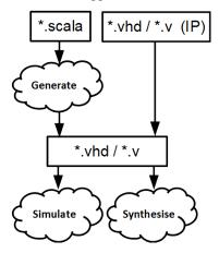
As SpinalHDL is interoperable with VHDL and (System)Verilog, you can both instantiate SpinalHDL IPs in these language (using generated code) and instantiate IPs in these languages in SpinalHDL (using BlackBox).
